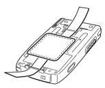
2. Fold the two ends of the hand strap back towards each other, and attach the fasteners as you adjust the length of the strap to fit your hand.
